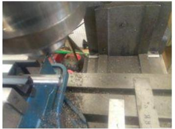
I cut a notch in the bottom of the barrel to clear the feed ramp on the magazine. It was .035 deep and .225 wide with .062 radius in the corners (.125 endmill)
