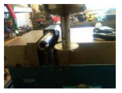
The extractor cut is centered vertically on the barrel.. Make the cut about twice as wide as your extractor, so it has plenty of clearance. You will cut into the rear of the chamber until you can see the extraction cannelure of a case thru the slot. Use the factory cut as a guide
