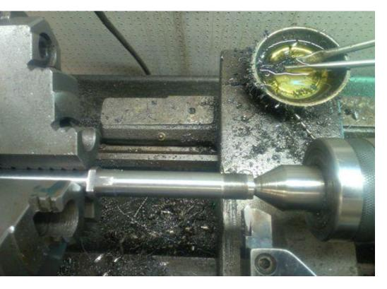
There is nothing significant about the .550 x 40 thread. I had a tap left over from when we made compensators for Springfield P9 Pistols. A suitable replacement could be  $9/16 \times 24$ , the small difference in diameter works out to about .005 per side, the single depth of 32 pitch thread is .020, so as long as you make the nut first and thread for close fit, it will be fine.
