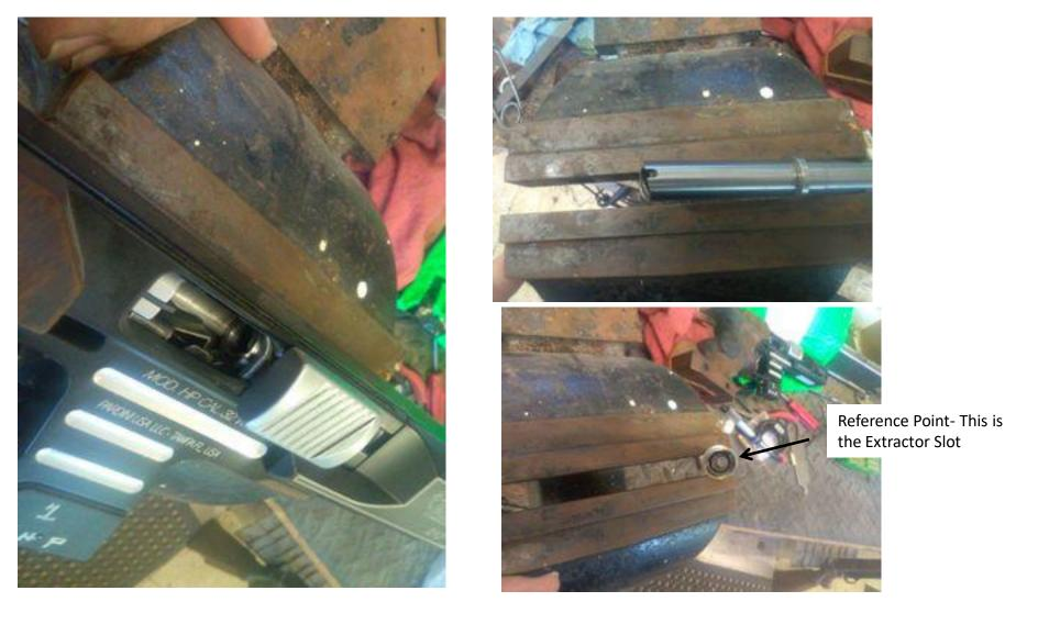
**FEED RAMP-** If you look closely you will see the feed ramp on the magazine is hooked under the barrel and will not allow the magazine to seat and lock. The factory addressed this with a large undercut on the barrel feed ramp.
