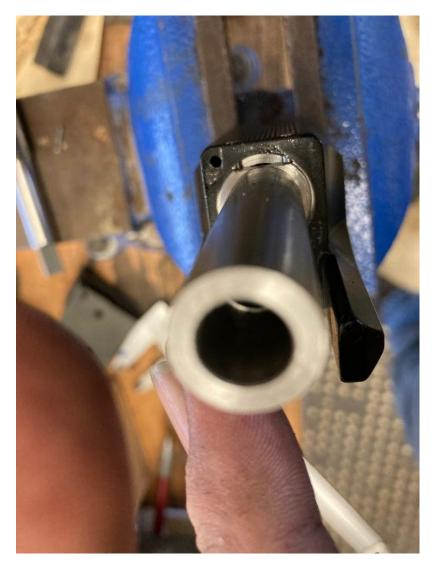
Install barrel in shroud and align flat with top of shroud. Insert pins with Loctite #270 and push them against flat on barrel. Set aside to cure.
