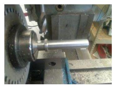
The barrel must index in the shroud to ensure the extractor cut and feed ramp are aligned correctly. I decided to install two (2) .093 dowel pins, .180 from center on each side, and cut a flat on the barrel to register on them. Pins were installed tangent to inner face of the flange cut. Flat on barrel was made tangent to .555 diameter on rear of barrel.
