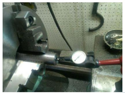
I had a 6 inch length of Krieger .308 1-10 twist barrel, left over from a rifle project. The barrel must be very carefully indicated for the least possible runout your lathe can provide. I read the groove, rather than the land, as my indicator gives better results that way. I was able to get it within .0002 total runout.
