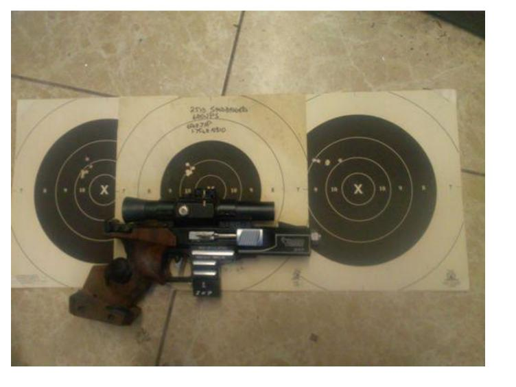
Here is the completed project with some test targets. Owner has much smaller hands than I do, so proper grip was a problem. The smallest group (center target) was the last fired, so I guess I got it figured out. Firing was done from sandbagged rest at 25yds. Please feel free to contact me with questions or comments, ask derrick@aol.com.
