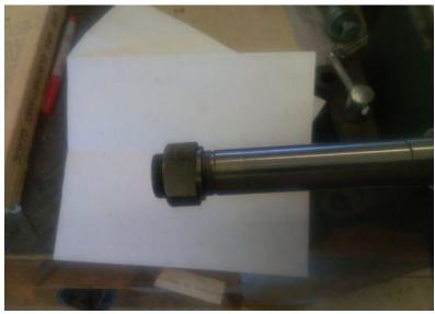
Here is the nut I made. Yours can be whatever you decide will work and looks good. If you decide to cut compensator slots into the barrel, be sure to leave it longer and slightly undersize (.005-.010 under root diameter) in front of the threads.
