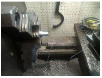
In the interest of concentricity and simplicity, I turned an aluminum rod to tightly fit the chamber. I could then drive it with friction on a live center and profile the entire barrel in one setup. Don't know if it's all that critical, but that's how I did it.
