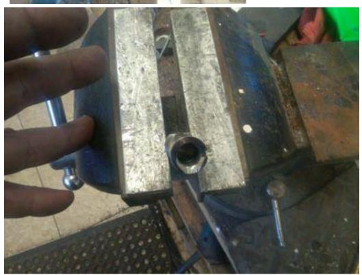
I then used 1/8 burr in MotoTool and cut small angles up the sides of the barrel and polished with cratex. Radius and polish the edges of the chamber to aid feeding. Next slide will give details on ammunition feeding.
