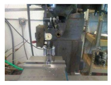
Here we are indicating the bore of the slide to ensure counterbore is correctly aligned.
