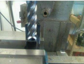
We now need to cut a recess in the shroud for the barrel flange. Indicate carefully and use a sharp ¾ inch endmill. Depth is .125 to match flange.
