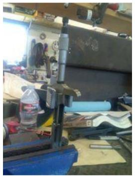
Time to check SAAMI against reality. The owner provided handloads he uses in the factory barrel, with new Hornady brass. I made a chamber gauge and measured the actual rim thickness, it was .045. Then I checked the factory rim cut in the slide (headspace) and found it was .054 (.009 over rim thickness). This means each time a round is chambered the firing pin has to drive it to the end of the chamber before it will fire. This would contribute to the owners accuracy issue.
